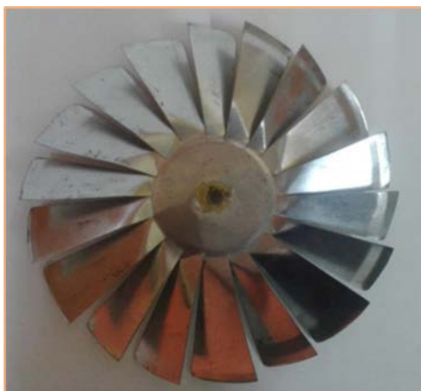
Fig. 3. Steam turbine consisted of 18 blades
